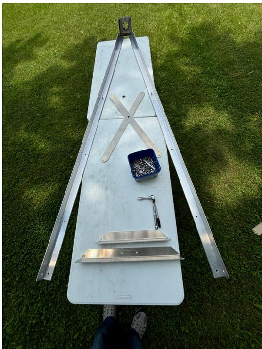
3. For the 810HD, assemble two legs and a top shelf collar bracket, together as shown in Figure 4.
