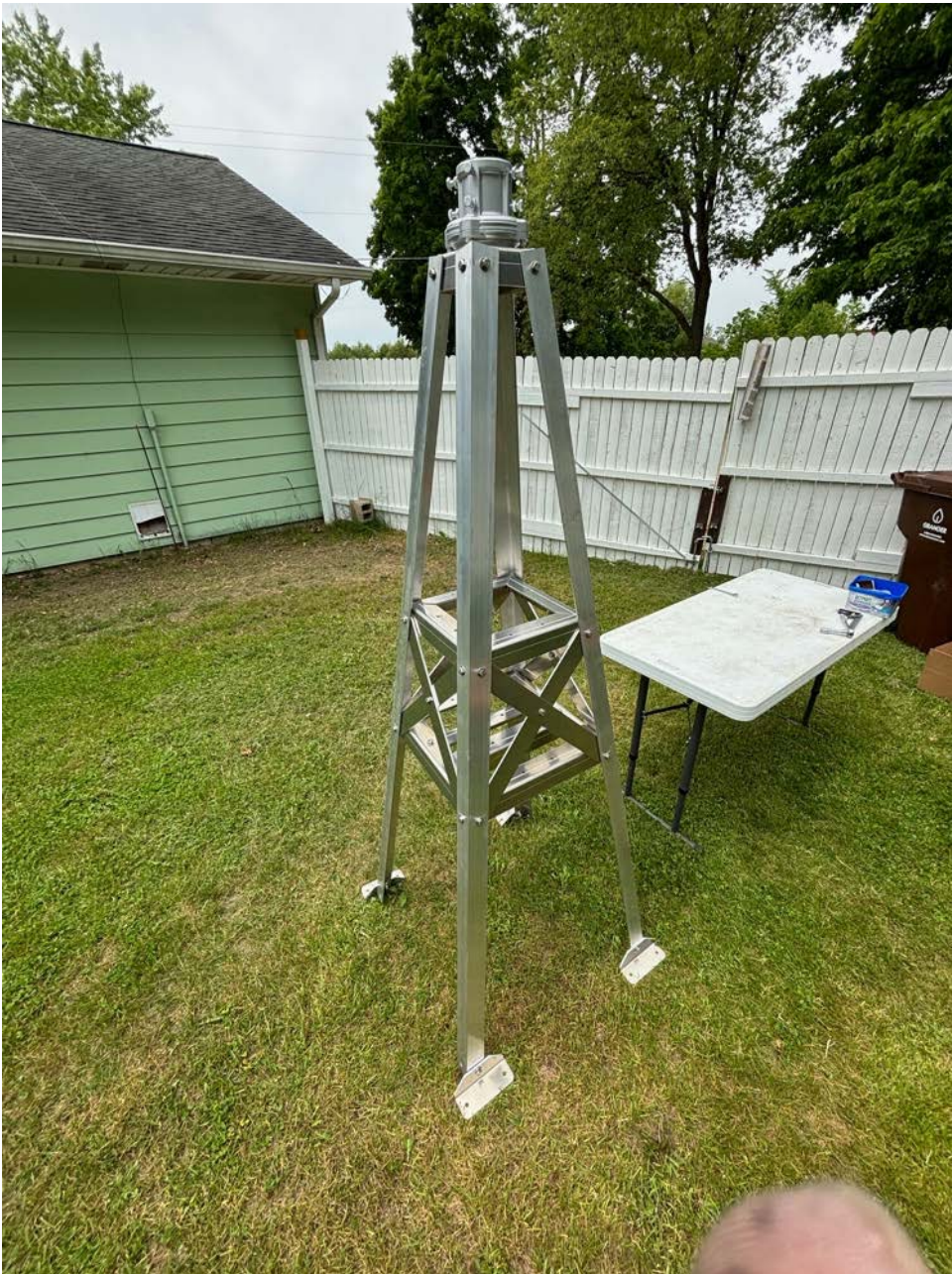
Figure 13 The finished 610HD Roof Tower Assembly.
